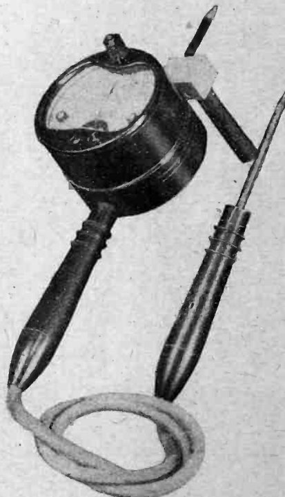
Ferranti cell-testing meter designed especially for cadmium tests.
